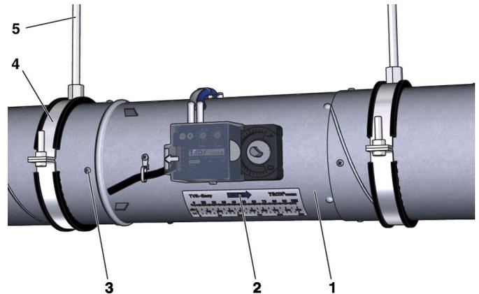
Fig. 9: Installation example using a VAV terminal unit TVR-\*
