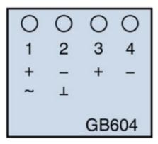
1  $\sim$ , +: Supply voltage 2  $\perp$ , -: Ground, neutral
