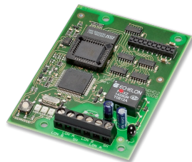
CENTRAL BMS INTERFACE
