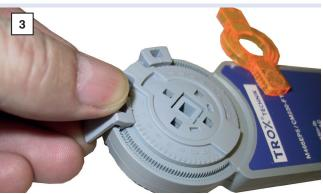
Remove the mechanical limiters
