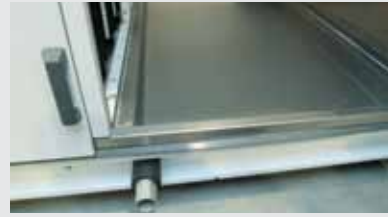
Stainless steel condensate drip tray, sloped in all directions, conforming to VDI 6022.
