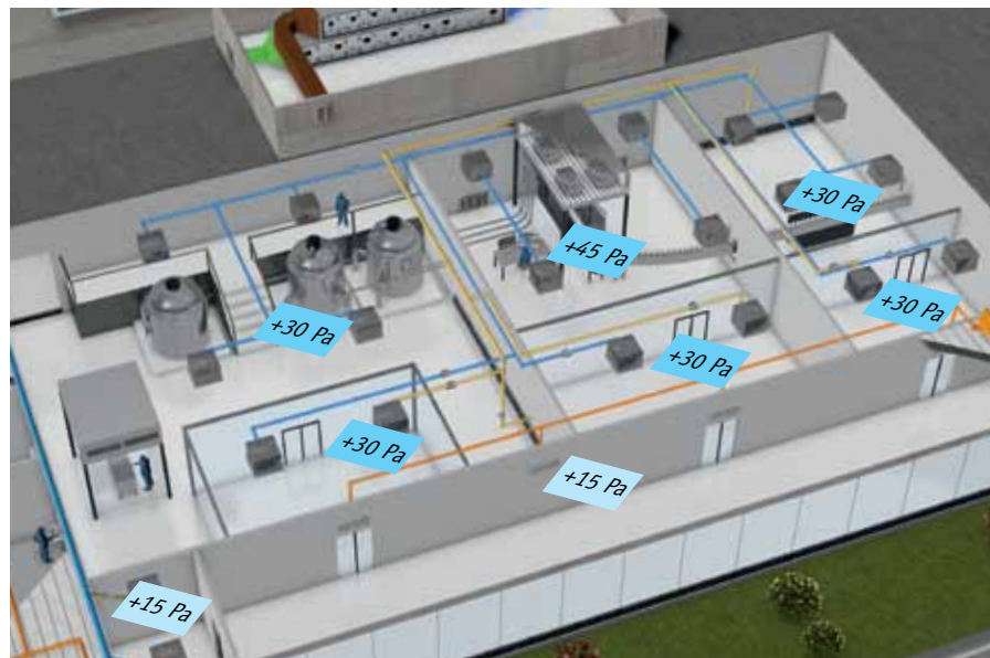
Critical areas can be isolated by means of precise pressure control and volume flow control.
